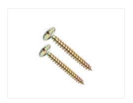
22x45 Washer Head Screw is a type of wide-head deep-threaded screw that is frequently preferred for drywall profile assemblies.
